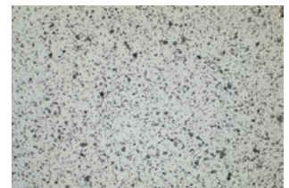
Ag/ZnO 92/8 SPW cross section
