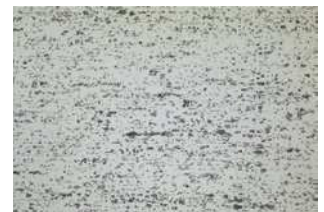
Ag/ZnO 92/8 SPW longitudinal section
